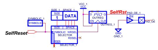
Figure 7. Self reset circuit using a Selector and one PIO pin, drawn in OrCAD Capture.
