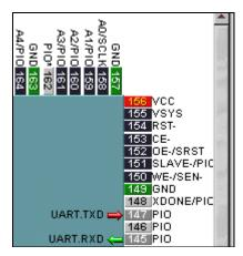
Figure 10. Place the UART TxD signal on pin 147. Place the RxD signal on pin 145.
