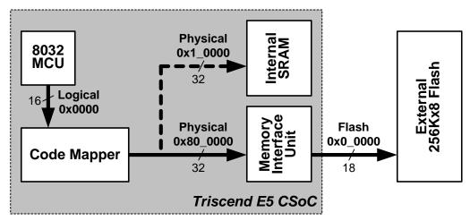
Figure 4. The 8032's 16-bit logic address is re-mapped to a 32-bit physical address space.
