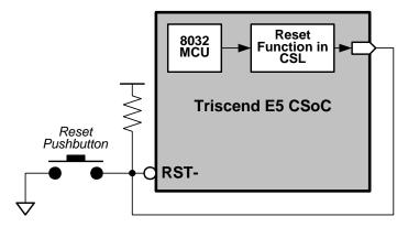
Figure 6. A Triscend E5 CSoC can reset itself using CSL/PIO circuitry.
