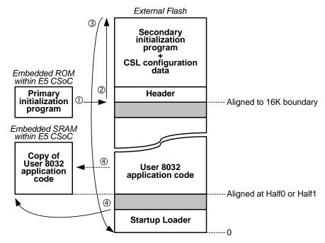
Figure 5. A modified initialization process supports secure Flash updates.
