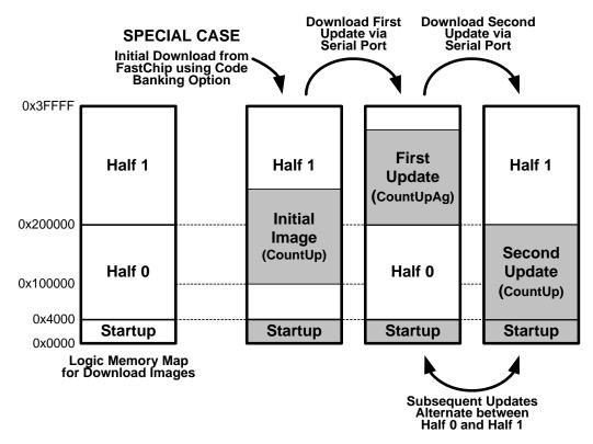
Figure 8. The Initial Download from FastChip is a special case. Subsequent updates are stored at either Half 0 or Half 1 in Flash memory.
