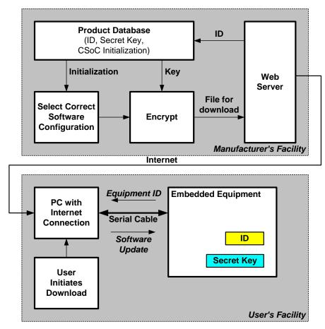
Figure 1. A potential software update architecture leveraging the world-wide web infrastructure. Simple approaches are possible using traditional phone lines or UARTs.
