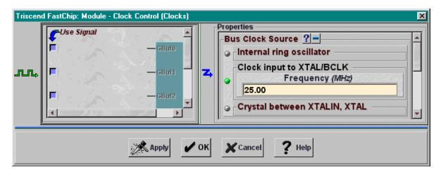
Figure 11. Configure the Bus Clock Source for BCLK and set the frequency to 25.00 MHz.
