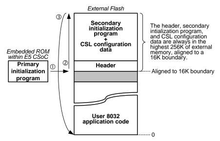
Figure 3. In a typical application, only a single initialization image is loaded from external Flash.
