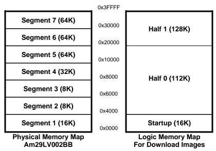
Figure 2. Subsequent updates are stored in either Half 0 or Half 1 in the Flash memory. The various Flash segments, with varying sizes, complicate the update software little.
