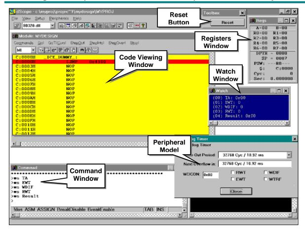
Figure 1. Keil dScope instruction-set simulator and debugger interface.
