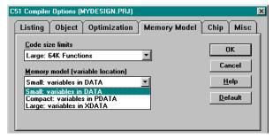
Always use the small memory model, unless the application will not fit or operate using the small model. The small model generates the fastest, tightest, and most efficient code. Variables within the application can always be explicitly specified to reside in other memory spaces.
