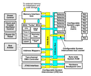
Figure 2. Triscend's E5 Configurable System on Chip Block Diagram
