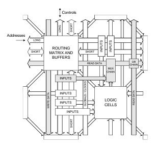
Figure 5. Signal flow in a Logic Tile
