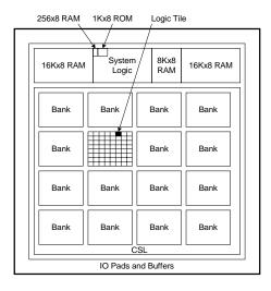
Figure 4. Physical Floor-plan of a Triscend E520
