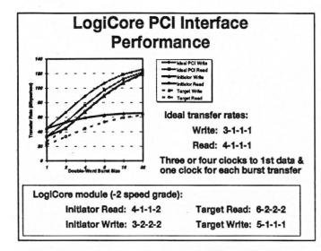
The chart compares the maximum data transfer rates for ideal PCI read and write operations and LogiCore PCI initiator and target transactions.
