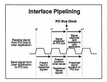
The LogiCore interface pipelines all of the bus control signals and the data path.
