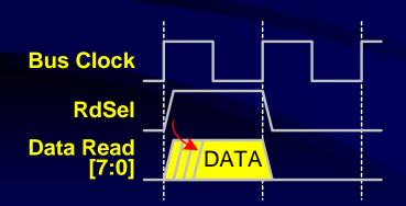
Decode delay is constant (less than 5 ns after clock)
