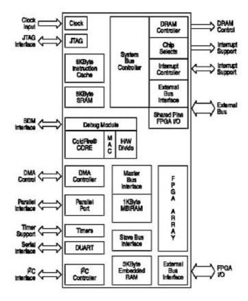
Figure 2. The CORE+ Configurable Processor based on Motorola's ColdFire processor. The CORE+ project died along with Motorola's MPA FPGA family [4].
