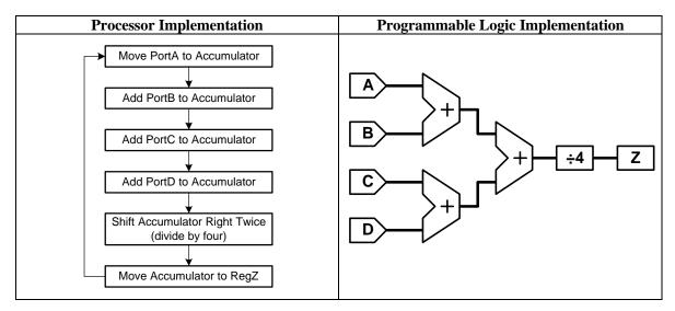
Figure 4. Two methods to compute the average of four incoming data values—one using a processor, the other using programmable logic. A Configurable Processor allows various hardware/software trade-offs.
