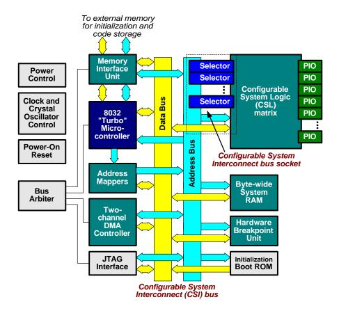
Figure 1. A block diagram showing the functions available within the Triscend E5 configurable processor. In the E5, the embedded 8032 "Turbo" microcontroller communicates to its programmable logic resource (CSL) via a dedicated internal bus structure [1].
