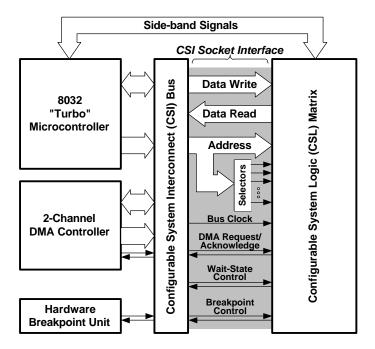
Figure 5. The Configurable System Interconnect (CSI) distributes address, data, control signals, and address decoding to the programmable logic resource (called the Configurable System Logic) in the Triscend E5 Configurable Processor.
