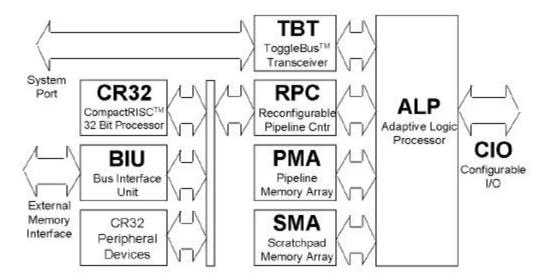
Figure 3. National Semiconductor's NAPA1000 configurable processor is a product of DARPA research funding [6].
