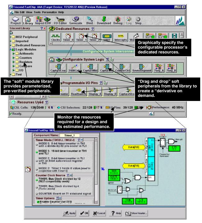
Figure 7. Defining the configurable processor hardware using the Triscend FastChip Development System. Standard peripheral functions can be loaded from the "soft" module library. Dedicated resources are also specified graphically.
