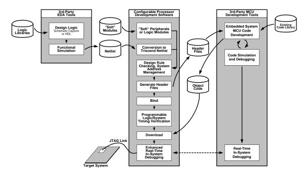
Figure 6. Detailed configurable processor design flow. Designers create a custom processor derivative using pre-defined "soft" modules. User can also create custom peripherals using schematic capture or logic synthesis design tools.
