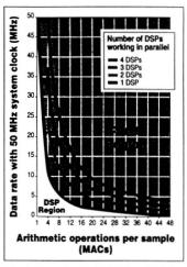
Chart shows in which situations FPGAs are suitable for DSP implementation.
