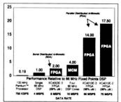
FPGAs can outperform traditional fixed-point DSP devices.
