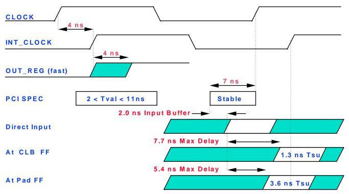
Figure 5. PCI and XC3100A-2 I/O timing.
