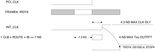
Figure 7. Handshake critical path.
