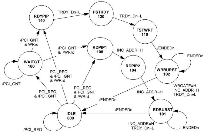
Figure 4. PIPCON State Diagram.
