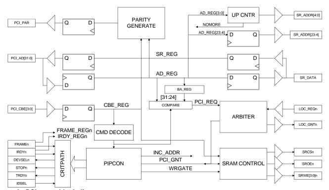
Figure 2. PCI target block diagram.
