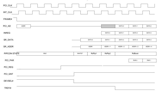
Figure 6. Read-cycle data flow.
