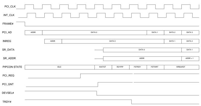
Figure 3. Write-cycle data flow.
