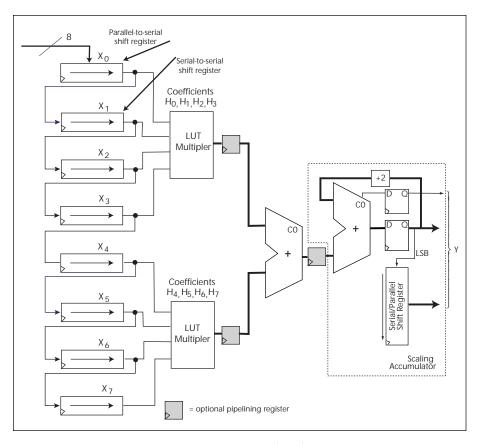
Fig 2—With the serial-distributed arithmetic (SDA) approach, the filter in Fig 1 becomes faster because this scheme determines the result in a scaling accumulator. This alternative cuts the number of constant-coefficient multipliers in half.
