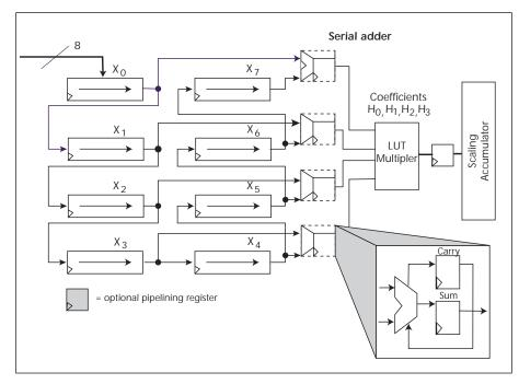
Fig 3—By turning the design of Fig 2 into a linear-phase filter, which has symmetrical coefficients, the implementation becomes somewhat simpler and requires one extra clock cycle.
