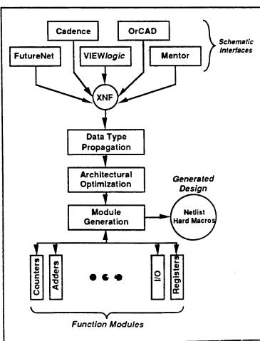
Figure 1. A block diagram of the Xilinx BLOX module generation system showing the significant elements.
