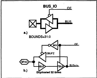
Figure 3. a.) A 32-bit bidirectional data bus specified with a single module symbol is much easier than drawing 32 gate-level representations as shown in b.).
