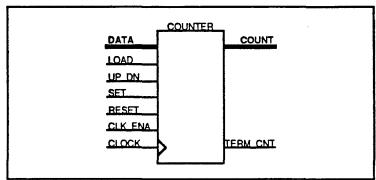
Figure 2. The COUNTER module from the Xilinx BLOX module library.
