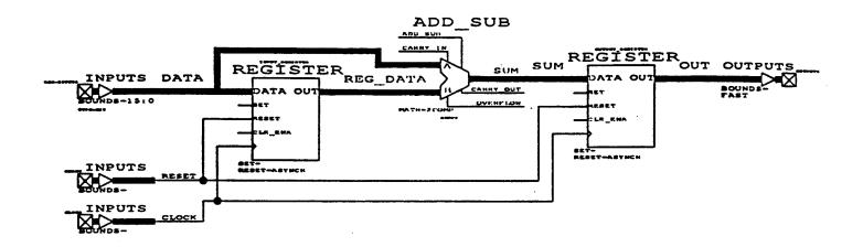
Figure 4. A complete design for a 16-bit registered adder drawn in VIEWlogic with Xilinx BLOX modules. The width and types for all data paths is automatically propagated throughout the design. The logic functions are generated and optimized for Xilinx XC4000 Field Programmable Gate Arrays.
