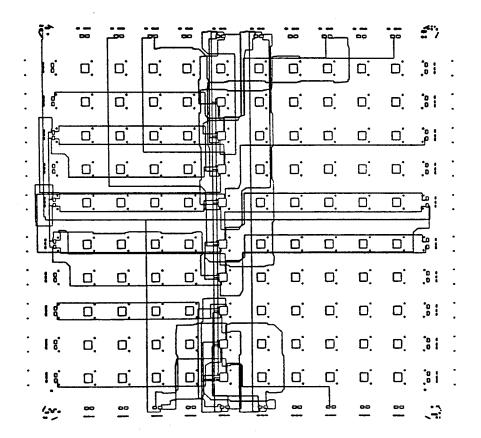
Figure 5. The same 16-bit adder design implemented in a Xilinx XC4003 device. The entire design occupies only a fraction of the available device resources. After the schematic diagram was entered, the design was automatically processed through the Xilinx software in under five minutes on a Sun® SPARCstation®.
