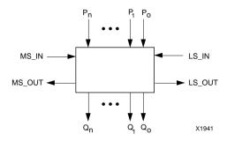
Figure 4-34 The Shift Register Data Flow Diagram
