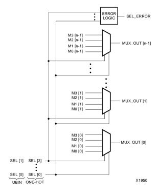
Figure 4-28 The 4-to-1 Bus-Multiplexer Logic Diagram
