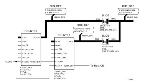
Figure 4-16 Cascading Counters without an Initial Clock Enable
