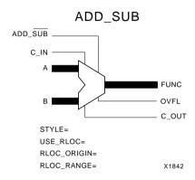
Figure 4-3 The Adder/Subtracter Module Symbol
