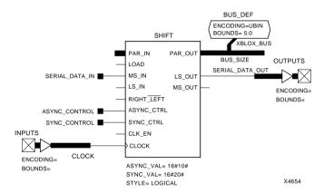
Figure 4-6 Serial-in/Serial-out Shift Register Using a BUS\_DEF Module to Define Its Data Type
