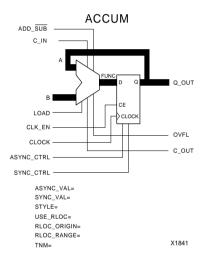
Figure 4-2 The Accumulator Module Symbol
