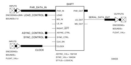
Figure 4-37 Typical Parallel-in/Serial-out Shift Register
