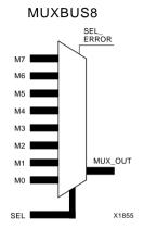
Figure 4-29 The 8-to-1 Bus-Multiplexer Module Symbol
