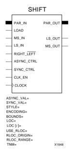
Figure 4-33 The SHIFT Module Symbol
