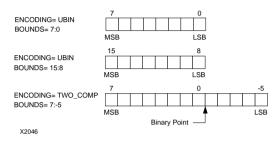
Figure 2-5 Example of BOUNDS and ENCODING Representation
