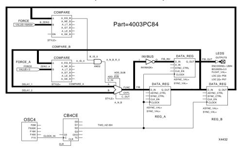
Figure 3-2 Sample Design — Fibonacci Sequence Generator Using the X-BLOX Design Tool
