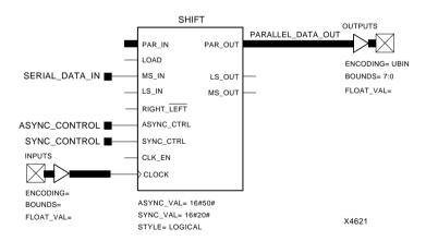
Figure 4-35 Typical Serial-in/Parallel-out Shift Register
