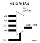
Figure 4-27 The 4-to-1 Bus-Multiplexer Module Symbol
