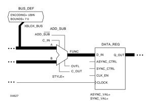
Figure 2-7 Simple X-BLOX Data Path Definition
