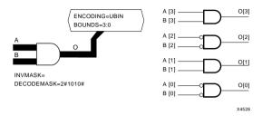
Figure 2-2 ANDBUS2 Using DECODEMASK
