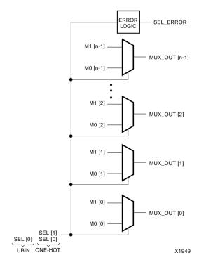
Figure 4-26 The 2-to-1 Bus-Multiplexer Logic Diagram
