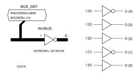
Figure 2-4 5-Input INVBUS Using INVMASK
