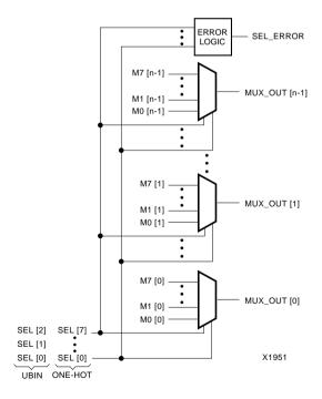
Figure 4-30 The 8-to-1 Bus-Multiplexer Logic Diagram
