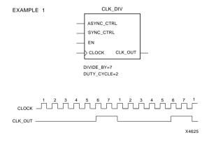
Figure 4-12 Simple Clock Divider Example
