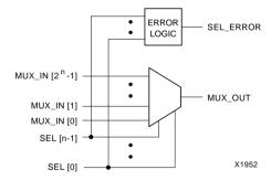
Figure 4-24 The n-to-1 Bus-Multiplexer Logic Diagram
