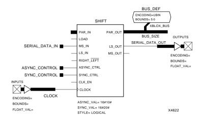
Figure 4-36 Typical Serial-in/Serial-out Shift Register
