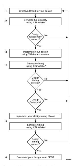
Figure 3-1 Incremental Design Flow
