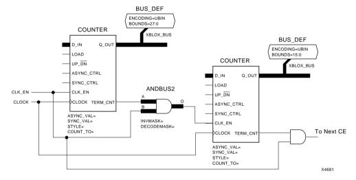
Figure 4-15 Cascading Counters with Clock Enable
