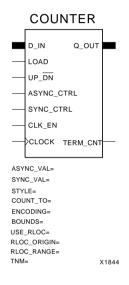
Figure 4-14 The Counter Module Symbol
