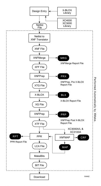
Figure 6-1 Implementation and Generation of a Bitstream File
